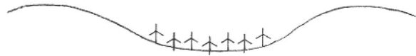
Fig 2: Wind energy development located in saddle between peaks – framing and, thus, accentuation achieved.
